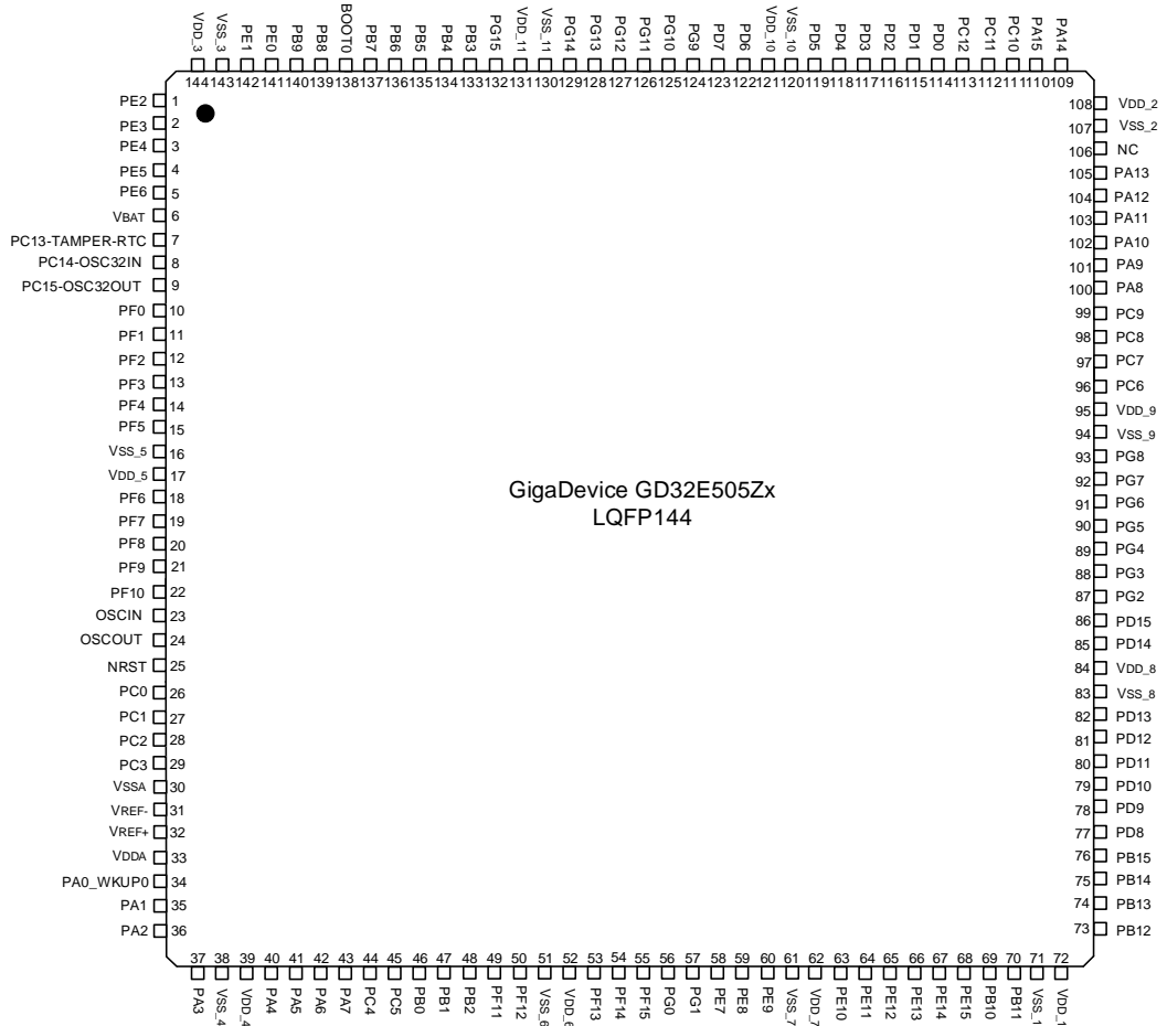
Figure 2-2. GD32E505Zx LQFP144 pinouts
