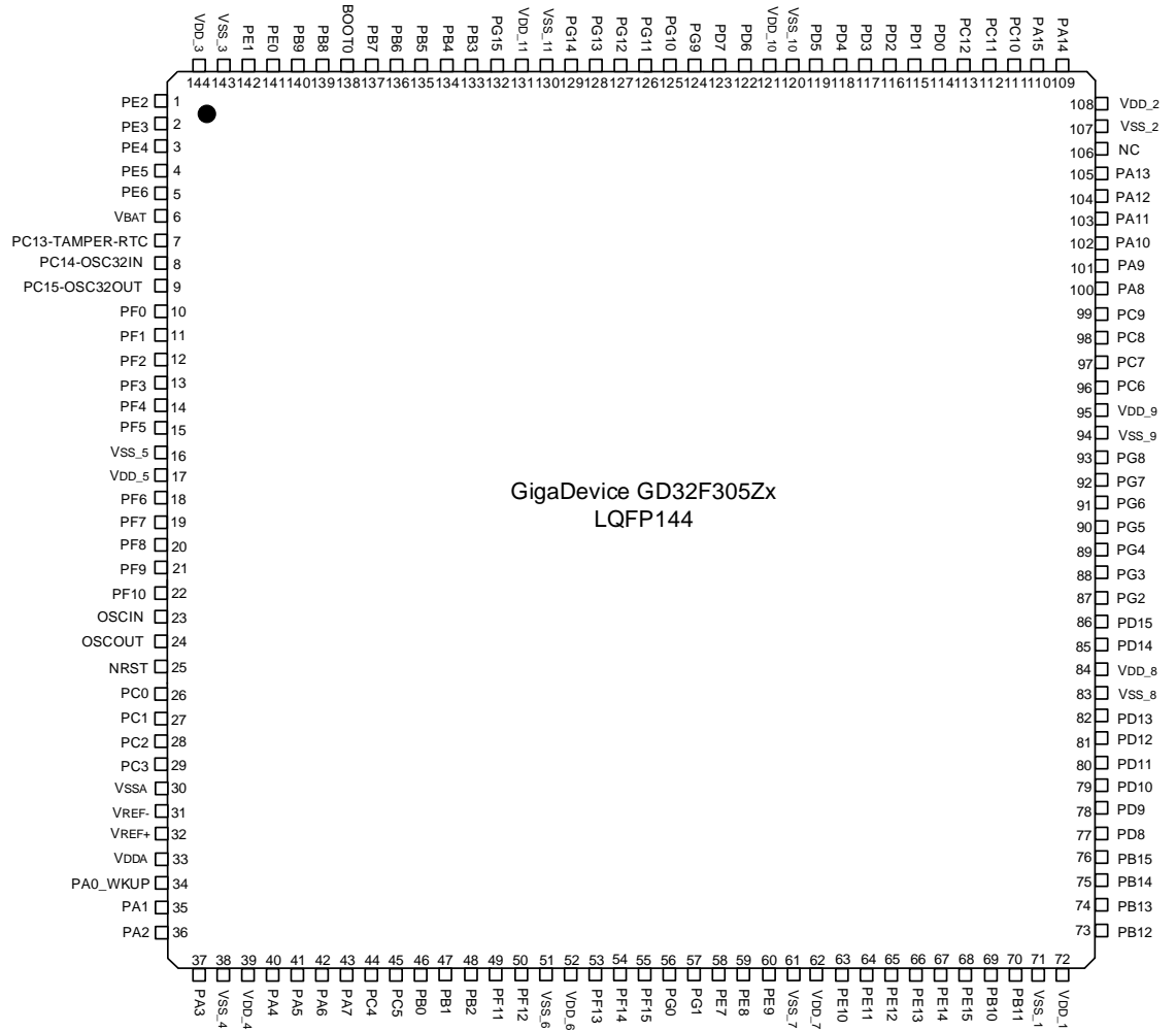
Figure 2-2. GD32F305Zx LQFP144 pinouts
