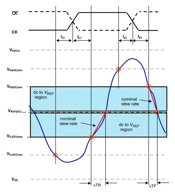
$$\frac{\text{Hold Slew Rate}}{\text{Rising Signal}} = \frac{V_{\text{REF(dc)}} - V_{\text{IL(dc)}} \text{max}}{\Delta \text{TR}} \quad \frac{\text{Hold Slew Rate}}{\text{Falling Signal}} = \frac{V_{\text{IH(dc)}} \text{min} - V_{\text{REF(dc)}}}{\Delta \text{TF}}$$
