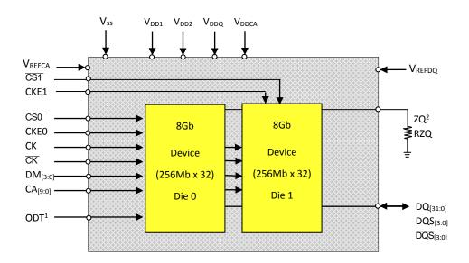
NOTE 1 ODT will be connected to rank0 (die0). The ODT input to rank1 (die1) will be connected to VSS in the package.
