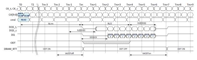
NOTE 1 The automatic RTT turn-off delay, tAODToff, is referenced from the rising edge of "RL-2" clock at Tm-2.
