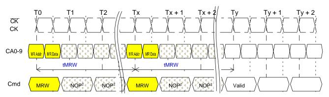
NOTE 1 At time Ty, the device is in the idle state.
