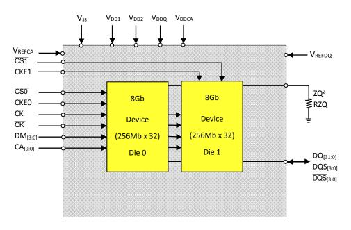
NOTE 1 ODT pins are NOT supported. ODT die pad is connected to VSS inside the package.
