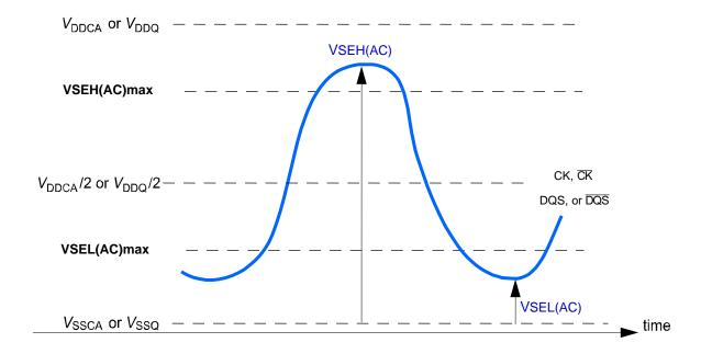
Note that while CA and DQ signal requirements are with respect to Vref, the single-ended components of differential signals have a requirement with respect to  $V_{DDQ}/2$  for DQS,  $\overline{DQS}$  and  $V_{DDCA}/2$  for CK,  $\overline{CK}$ ; this is nominally the same.
