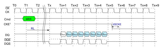
NOTE 1 CKE can be registered LOW RL + RU(tDQSCK/tCK)+ BL/2 + 1 clock cycles after the clock on which the MRR command is registered.
