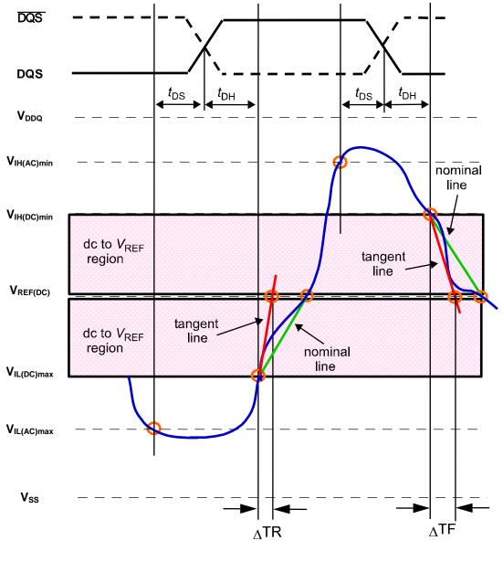
tangent line [  $V_{REF(dc)} - V_{IL(dc)} max$  ] Hold Slew Rate Rising Signal ΔTR
