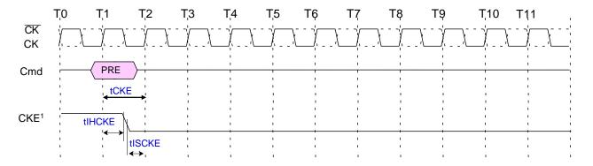
NOTE 1 CKE can go LOW tIHCKE after the clock on which the PRECHARGE command is registered.
