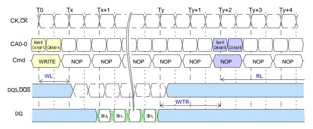
NOTE 1 The minimum number of clock cycles from the burst WRITE command to the burst READ command for any bank is [WL + 1 + BL/2 + RU(tWTR/tCK)].
