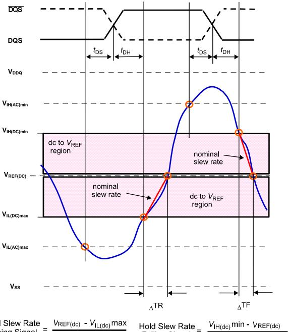
$$\begin{array}{c} \text{Hold Slew Rate} \\ \text{Rising Signal} = \frac{V_{\text{REF(dc)}} - V_{\text{IL(dc)}} \text{max}}{\Delta^{\text{TR}}} & \text{Hold Slew Rate} \\ \text{Falling Signal} = \frac{V_{\text{IH(dc)}} \text{min} - V_{\text{REF(dc)}}}{\Delta^{\text{TF}}} \end{array}$$
