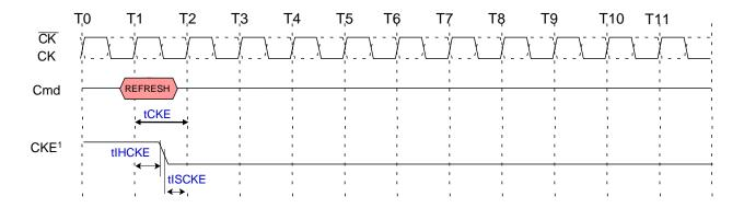
NOTE 1 CKE can go LOW tIHCKE after the clock on which the REFRESH command is registered.
