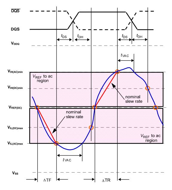
Setup Slew Rate Falling Signal =
