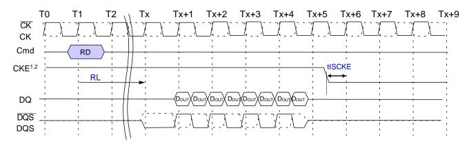
NOTE 1  $\,$  CKE must be held HIGH until the end of the burst operation.
