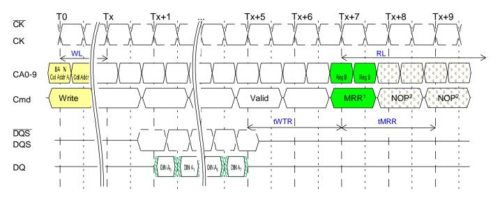
NOTE 1 The minimum number of clock cycles from the burst WRITE command to the MRR command is [WL + 1 + BL/2 + RU(tWTR/tCK)].
