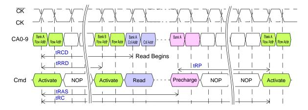
NOTE 1 A PRECHARGE-all command uses tRPab timing, while a single-bank PRECHARGE command uses tRPpb timing. In this figure, tRP is used to denote either an all-bank PRECHARGE or a single-bank PRECHARGE.
