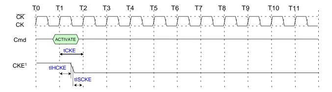
NOTE 1 CKE can go LOW tIHCKE after the clock on which the ACTIVATE command is registered.
