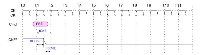
NOTE 1 CKE can go LOW tIHCKE after the clock on which the PRECHARGE command is registered.
