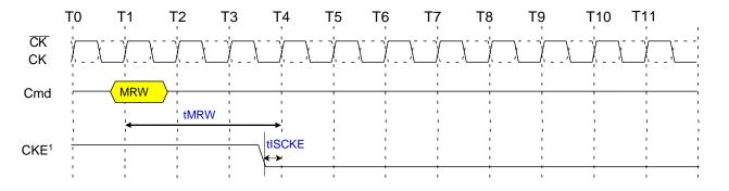
${\tt NOTE~1} \quad {\tt CKE~can~be~registered~LOW~tMRW~after~the~clock~on~which~the~MRW~command~is~registered}.$
