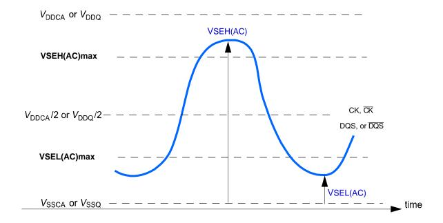
Note that while CA and DQ signal requirements are with respect to Vref, the single-ended components of differential signals have a requirement with respect to V<sub>DDQ</sub>/2 for DQS, DQS and V<sub>DDCA</sub>/2 for CK, CK; this is nominally the same.
