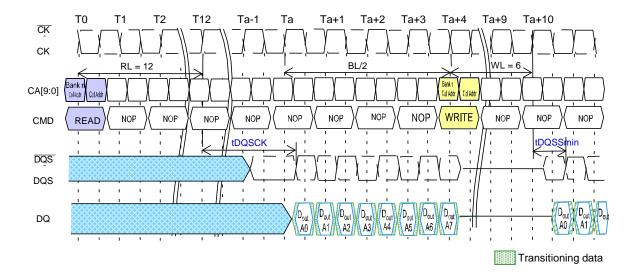
The minimum time from the burst READ command to the burst WRITE command is defined by the read latency (RL) and the burst length (BL). Minimum READ-to-WRITE latency is RL + RU(tDQSCK(MAX)/tCK) + BL/2 + 1 - WL clock cycles.
