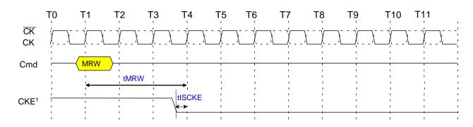
NOTE 1 CKE can be registered LOW tMRW after the clock on which the MRW command is registered.
