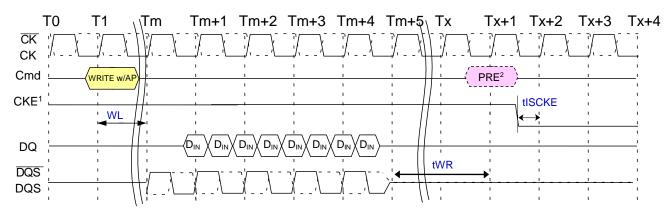
NOTE 1 CKE can be registered LOW at WL + 1 + BL/2 + RU(tWR/tCK) + 1 clock cycles after the WRITE command is registered. NOTE 2 Start internal PRECHARGE.
