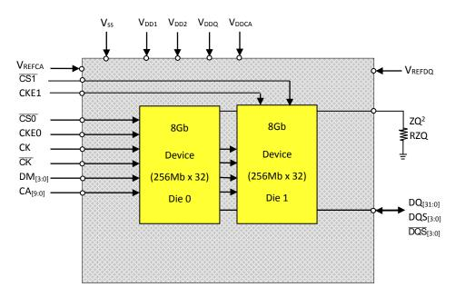
NOTE 1 ODT pins are NOT supported. ODT die pad is connected to VSS inside the package.
