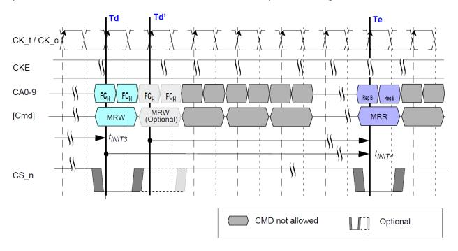
NOTE 1 Optional MRW RESET command and optional  $\overline{CS}$  assertion are allowed, When optional MRW RESET command is used, *t*INIT4 starts at Td'.
