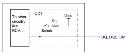
The switch is enabled by the internal ODT control logic, which uses the external ODT pin and other mode register control information. The value of *R*TT is determined by the settings of mode register bits.
