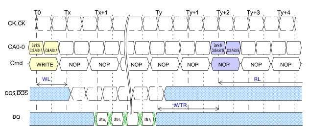
NOTE 1 The minimum number of clock cycles from the burst WRITE command to the burst READ command for any bank is [WL + 1 + BL/2 + RU(tWTR/tCK)].
