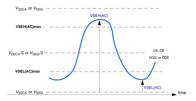
Note that while CA and DQ signal requirements are with respect to Vref, the single-ended components of differential signals have a requirement with respect to  $V_{DDQ}/2$  for DQS,  $\overline{DQS}$  and  $V_{DDCA}/2$  for CK,  $\overline{CK}$ ; this is nominally the same.
