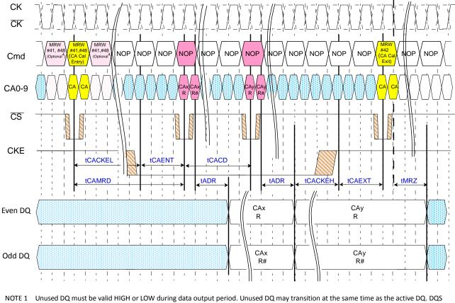
NOTE 1 Unused DQ must be valid HIGH or LOW during data output period. Unused DQ may transition at the same time as the active DQ. DQS must remain static and not transition.
