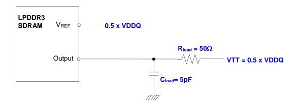
NOTE 1 All output timing parameter values (tDQSCK, tDQSQ, tHZ, tRPRE, etc.) are reported with respect to this reference load. This reference load is also used to report slew rate.
