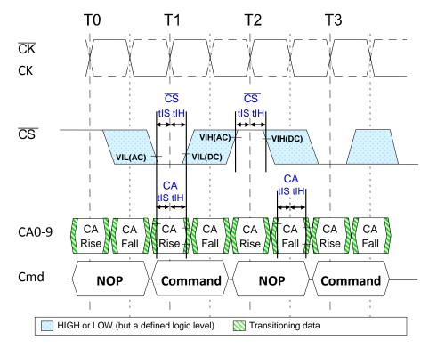
NOTE 1 Setup and hold conditions also apply to the CKE pin. For timing diagrams related to the CKE pin, see "Power-Down"
